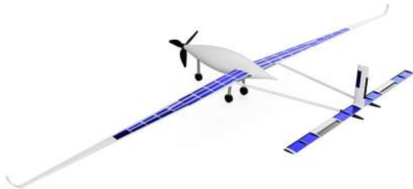
Figure 1. 3-D Solar powered UAV
